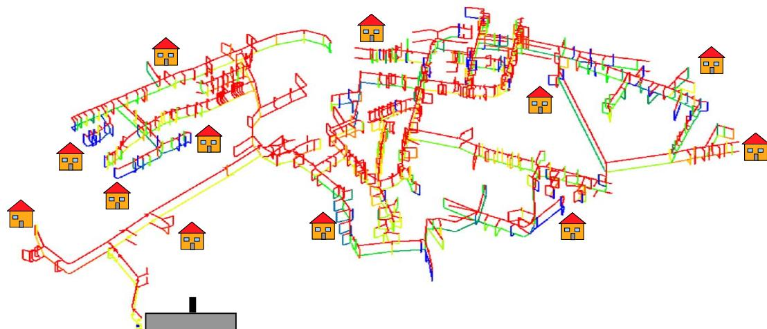
*Figure 1 Simulation model of the district heating grid of Rheinsberg/Germany. The simulation model includes also 500 simple dynamic building models and the corresponding heat transfer relay stations.*
