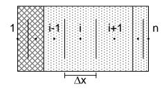
Figure 1 Control volumes and node structure
