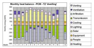
Figure 23 Monthly heat balance for the thermal zone 'dwelling' (variation 'PCM')
