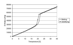
Figure 2 Enthalpy as a function of temperature
