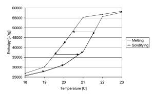
Figure 3 State of PCM. Sample melt/solidify loop
