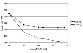
Figure 11 Energy use as a function of PCM area
