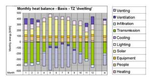
Figure 22 Monthly heat balance for the thermal zone 'dwelling' (variation 'Basis')
