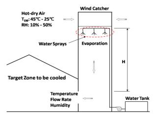
Figure 1 Schemetic of PDEC tower with spray
