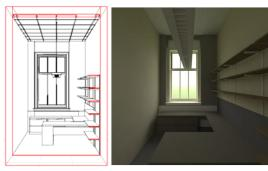
Figure 3 3D model and simulation of the office space with CIE overcast sky
