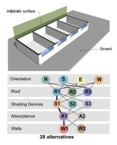
*Figure 13 – Model 3: generation of alternatives.*
