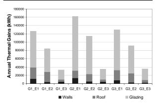
Figure 6 – Model 1: Annual thermal gains of simulated cases.
