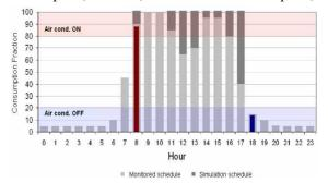
Figure 3 – Air conditioning schedules: hours when equipments are turned on and off.
