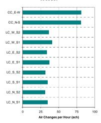
Figure 10 - Model 2: Air changes per hour
