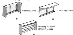
Figure 14 – Simulated shading devices.
