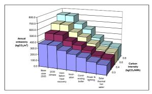
Figure 7. Effect of carbon intensity of grid electricity on emissions from newer hotel
