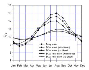
Figure 7 Comparsion of annual monthly mean water temperatures derived from a 2500m borefield and a 400m 4-well SCW cluster ('near earth' represents the earth condition at 1m from well centre)
