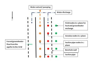
Figure 3 Cross section of the well model (the borehole and pipe wall resistances are omitted in this figure)
