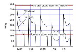
Figure 4 Simulated heating delivered by a cluster of 4 x 100m-deep SCWs operating at capacities within the range of that reported by Orio et al. (2005)
