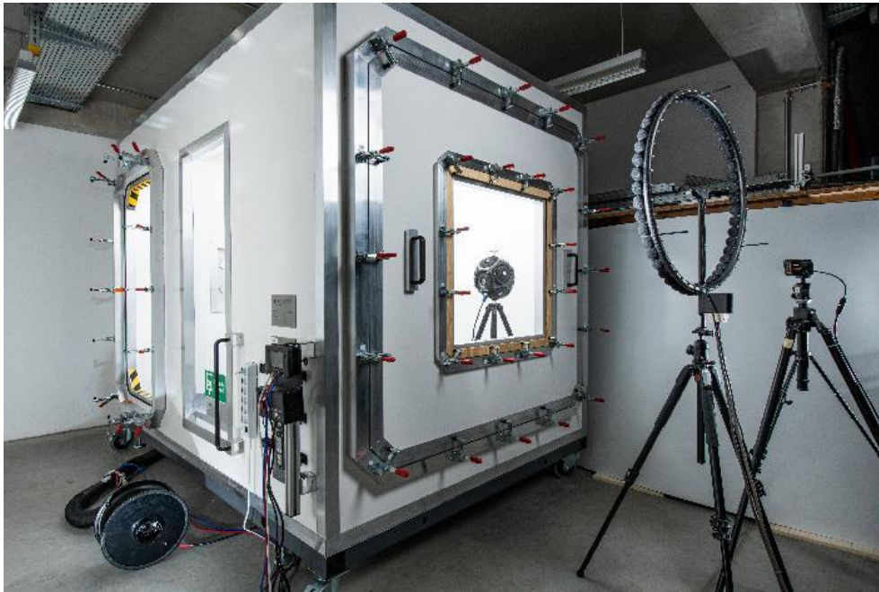
Figure 33: Test facility ATLAS equipped with its requisite measurement technology: Minneapolis DuctBlaster with Micro Leakage Meter (left), loudspeaker (inside), microphone array (right) and infrared camera (right) (Diel, Schiricke, & Pernpeintner, 2024)
