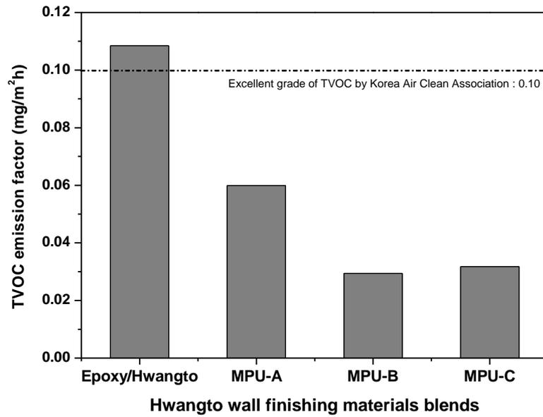
**Fig. 1** TVOC emission of Hwangto wall finishing materials blends
