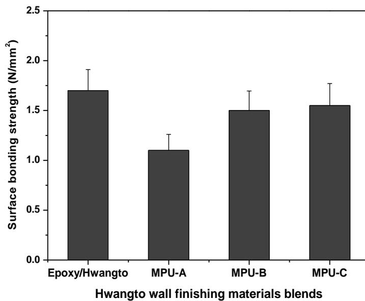
**Fig. 2** Surface bonding strength of Hwangto wall finishing blends
