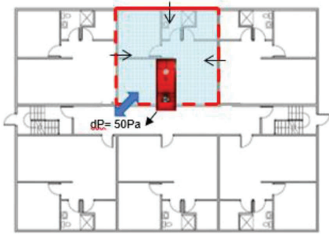
Figure 6. Compartmentalization test of single unit in a common-entry bi
