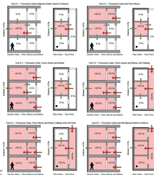
Figure 6.5: Balanced Fan Pressurization/Depressurization Method Schematic (Finch, 2009)
