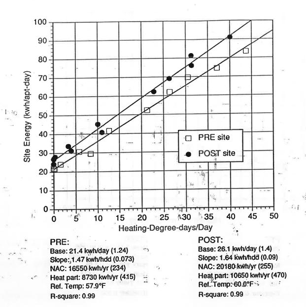
Figure & Weather-normalized energy consumption, pre- and post-retrofit.
