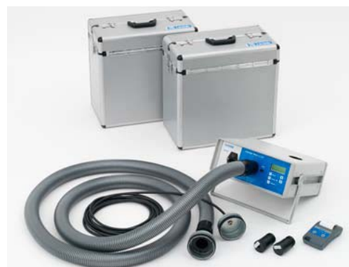
Figure 20 Another example of Swedish duct leakage testing equipment [Lindab]
