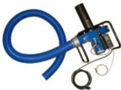
Figure 19 Example of Swedish duct leakage testing equipment [Swema]
