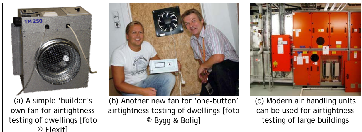
Figure 12: Examples of products for simple testing of airtightness
