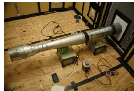
(b) Air-leakage tester
