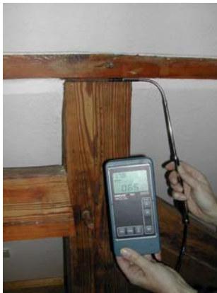
Figures 3,4,5: Draughts at the joint between post and center purlin (0.65 m/s); flow through the ceiling (air flow rate at the ceiling opening 3.4 m/s) due to incomplete airtight layer at the ceiling joint
