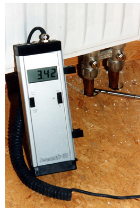
Figures 3,4,5: Draughts at the joint between post and center purlin (0.65 m/s); flow through the ceiling (air flow rate at the ceiling opening 3.4 m/s) due to incomplete airtight layer at the ceiling joint
