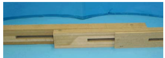
Figure 3: Slot typeB:- Fixed height, varying depth
