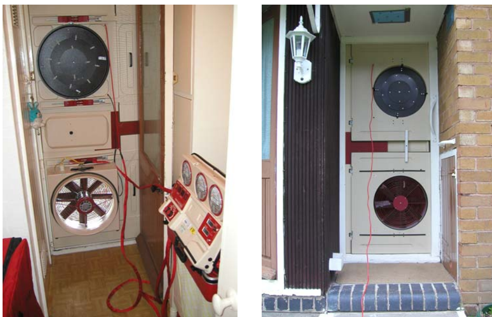
Figure 1: Internal and external view of blower door
