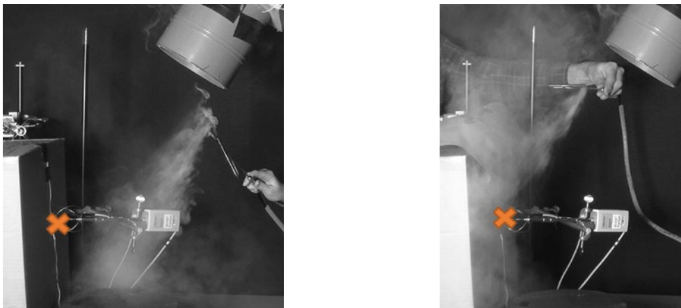
Figure 3 Visualization of the air stream caused by the PV system. Left: smoke supplied from the front, Right: smoke supplied from the back. Orange cross: breathing zone.
