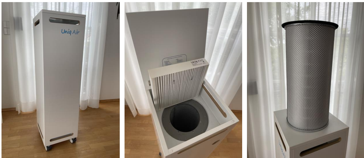
Figure 1 Foto of mobile air cleaner UniqAir PRO (left); G4 pre-filter and view on cylindrical H13 filter flange (middle); cylindrical H13 filter with inner layer of active carbon (right)
