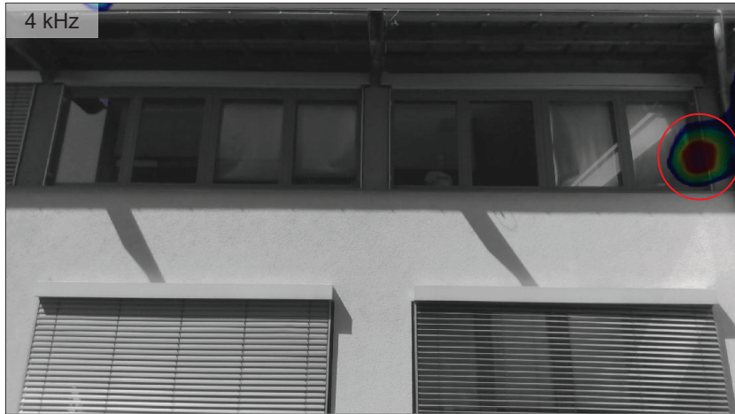
Window seals are damaged
