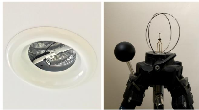
Figure 4 T/RH sensor in supply vent (left) and PMV experimental probe and sensor (right)
