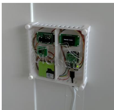
Figure 2: Example of mounted measurement device (in 3D-printed housing)
