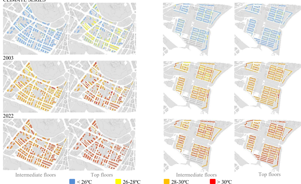
Figure 4. GIS plan with maximum average indoor operative temperature in August for 2022 weather files considering microclimate (left: N1; right: N2)
