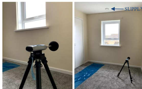
Figure 3 Experimental set-up using Pulsar Nova 46 sound level meter
