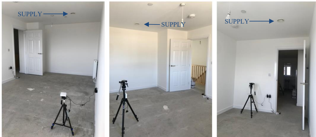
Figure 2 Tracer gas set-up in rooms of different sizes and layout
