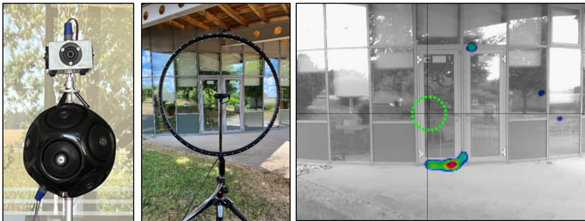
Figure 2: Measurement setup: pair of loudspeakers inside (left), microphone array or acoustic camera outside (centre), visualization of the loudest noise sources on the facade (right).
