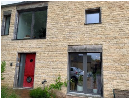
Figure 4: Blower door fan setup in a doorway and taped from inside
