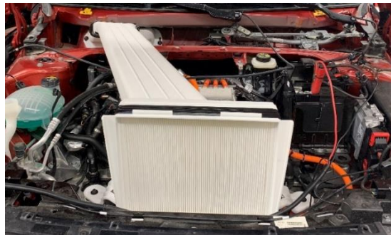
Figure 2 Pre-filter prototype installation in an existing production vehicle's thermal compartment
