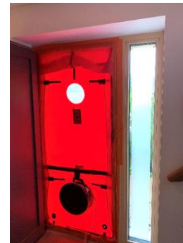
Figure 4: Blower door fan setup in a doorway and taped from inside
