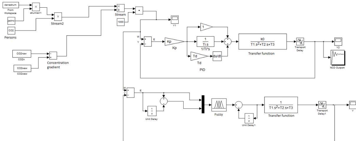
Figure 8. CO<sub>2</sub> concentration control model with classical PID control and PI fuzzy control.
