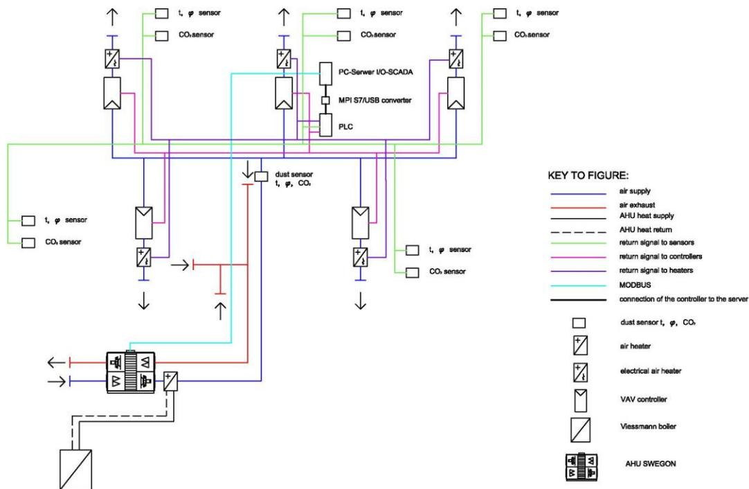
Figure 12. Symbolic diagram of a modernized system with all measurement devices, actuators and control
