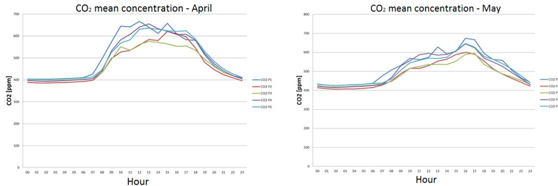
Figure 13. Daily changes of CO<sub>2</sub> concentration in each of the controlled spheres of a passive building: April (a) and May (b).
