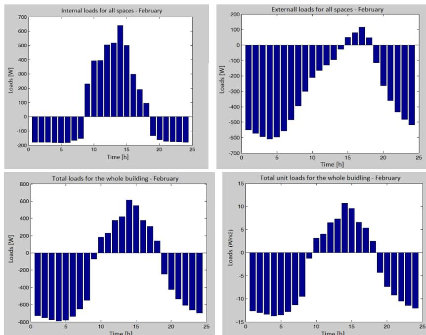
Figure 6. example of loads (for February) for a passive building under test:
