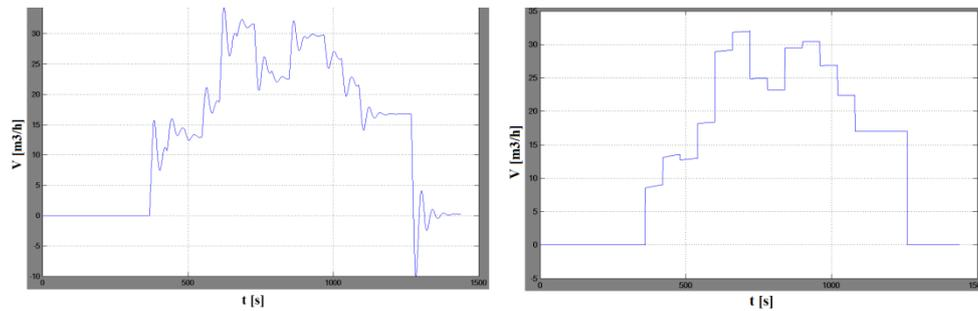
Figure 9. Setting the optimal air stream based on the CO<sub>2</sub> concentration balance (a) and the result of the simulation of the requested air stream control with a PID controller (b) and FLC Mamdani fuzzy controller (c).
