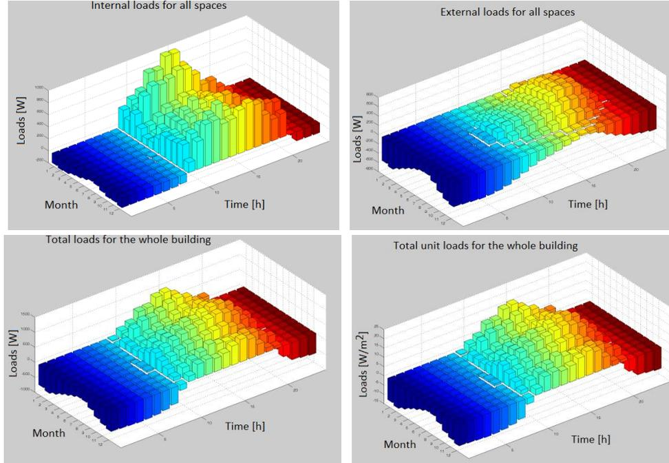
Figure 7. Daily loads of a passive building in question set for the whole year: a-internal, b-external, c-total, d-unit.
