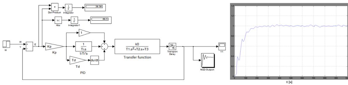
Figure 4. Model of the tested automatic control system with a PID-type controller (a) and the response of the control system as a simulation result (b).
