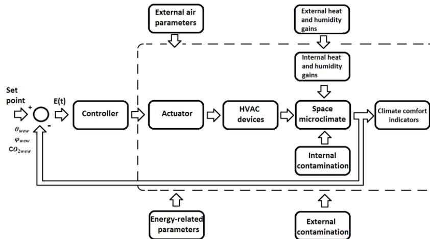
Figure 3: An example of an automatic climate comfort control system in passive and low-energy buildings.
