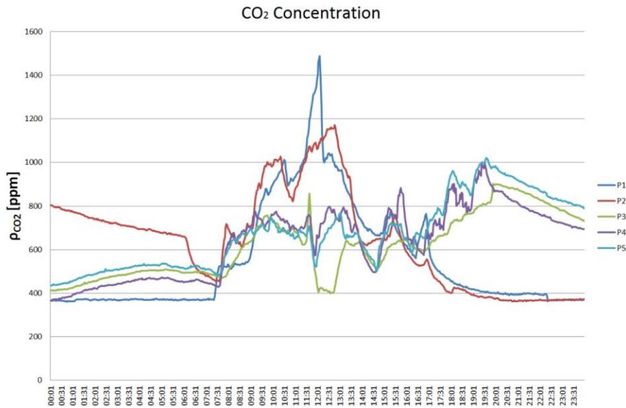
Figure 11. Example of daily changes of CO<sub>2</sub> concentration for each sphere (room)
