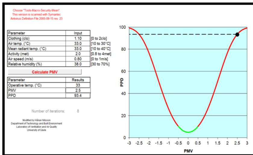
Figure 3: PMV calculation, (PMV calculation programme. Håkan Nilsson, Department of Technology and Built Environment)
