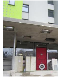
Setup in exterior door of ground floor
