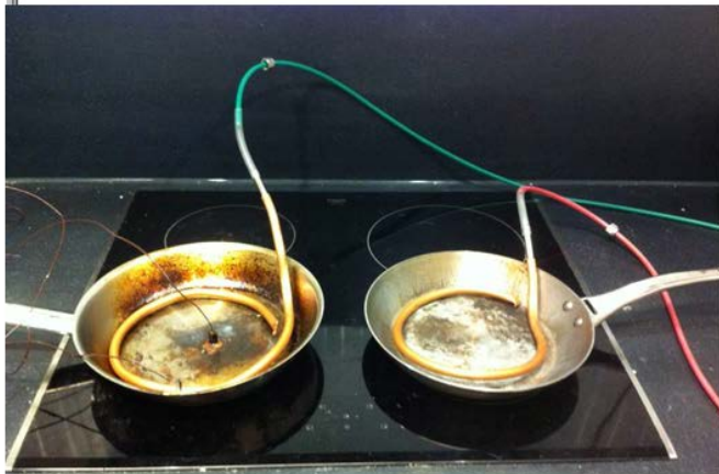
Figure 2. Induction method with \text{CO}_2 injection in two stainless steel 24-cm stir-fry pans in the front locations, the left pan is equipped with temperature sensors.
