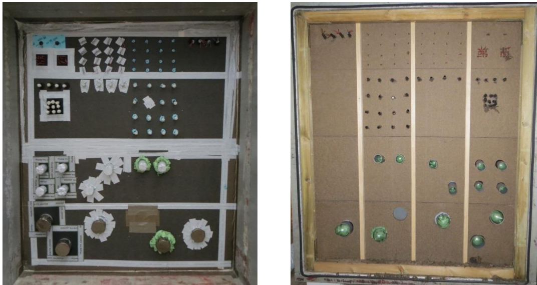
Figure 2: Wood-frame wall with different air sealing solutions in steel test rig
