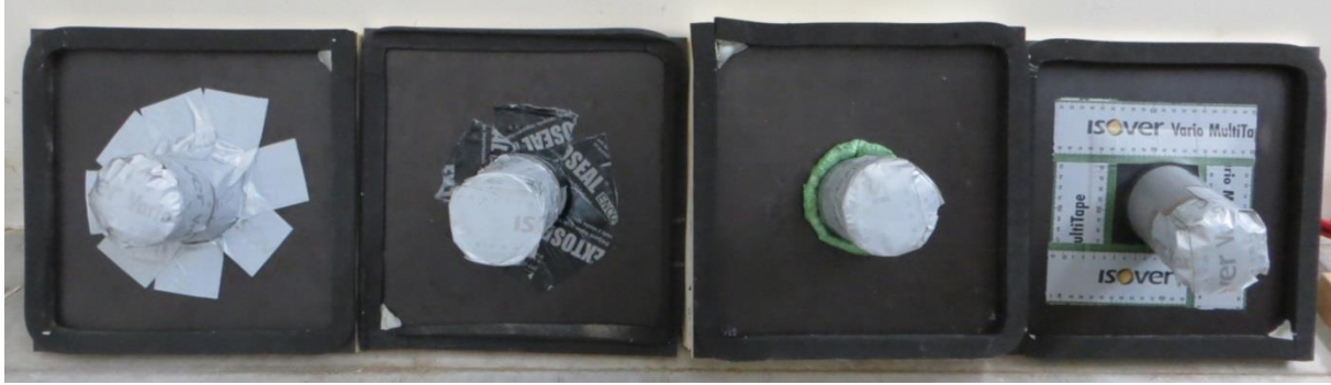
Figure 4: Test specimens: tape (1), tape (2), PUR, gasket
