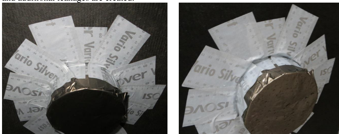
Figure 5: Durability effects taped PVC pipe: before and after water tightness testing
