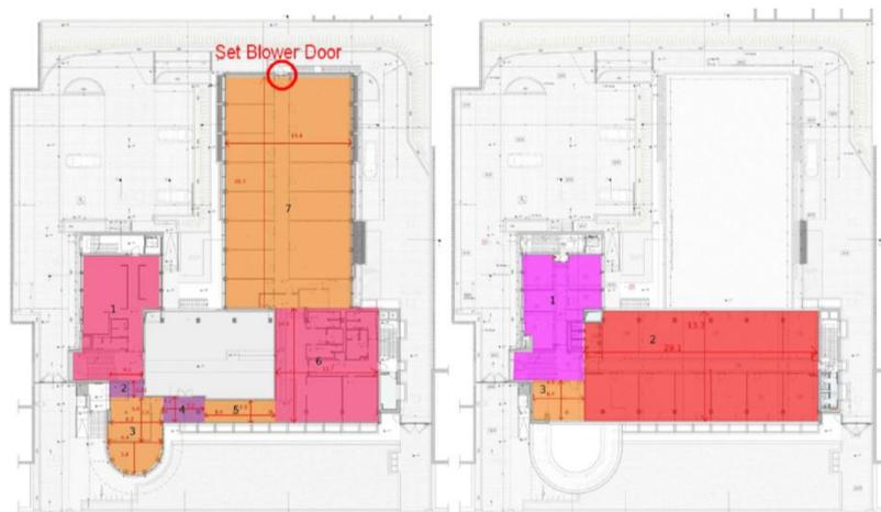
Figure 8: Building floors (left ground floor, right +1), coloured zones are part of the renovation project, taken from the test report (Delire et al., 2013)
