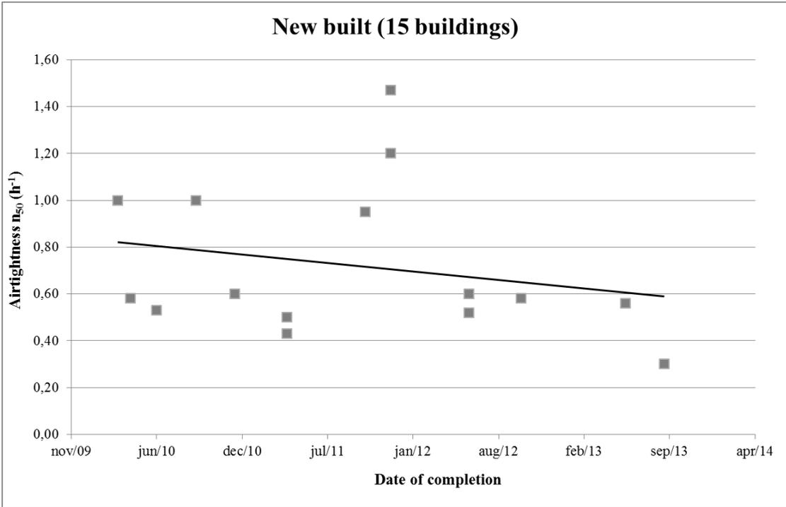
Figure 12: Evolution of airtightness of new built tertiary buildings in time, dataset of the Exemplary Buildings program
