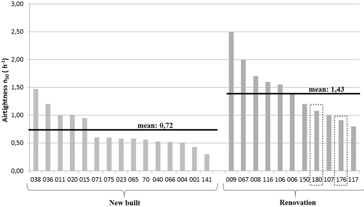
Figure 10: Range of measured building airtightness for new built and renovation in the Exemplary Buildings program. Case studies are indicated in the dotted boxes (case study EFH = number 176, Tritomas = number 180)
