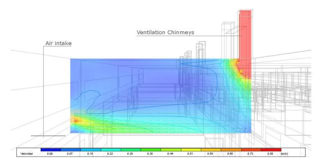
One of the objective of this study is to check the consumption of energy, besides the CO<sub>2</sub> emissions to the atmosphere, and these are lower in the Proposed Building using natural ventilation than in the Reference Building with mechanical ventilation and heat recovery, according to requirements of RITE.
