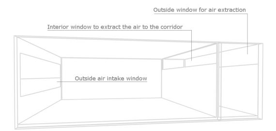
• 2 windows (one practicable + 1 fixed + ventilation shunts): The ventilation of the area is performed by opening the lower longitudinal window (air intake) and opening the vents of the shunts (exhaust air), which extract the air from the zone to the outside area by the ventilation chimneys on deck. The admission of outside air can be introduced by a strip as specified in the following illustration, or through openings to
