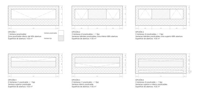
In addition to the different situations of the openings in the façade, two techniques for cross ventilation are evaluated. The first is achieved by arranging an opening in the top of the inner partition which separates each office with the corridor. And the second creating shunts and ventilation chimneys.
