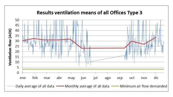
Air changes per hour are always above the minimum required, justifying the requirements of RITE. Thanks to the installation of motorized louvers in the openings to the outside, we can modulate the amount of air entering each zone, providing only the amount of the required air depending on the CO<sub>2</sub> concentration that exists in every area at every moment. The air flow pattern can be seen in the following image:
