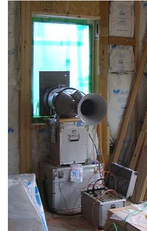
Figure 2. Measuring air tightness.
