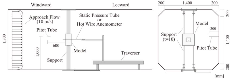
**Fig.3 Experimental set-up of the measurement along the central line**
