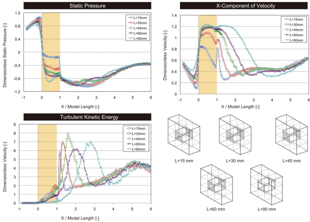
**Fig.6** Flow quantities along the central line of the openings
