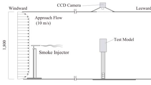
**Fig.4 Experimental set-up for PIV measurement**
