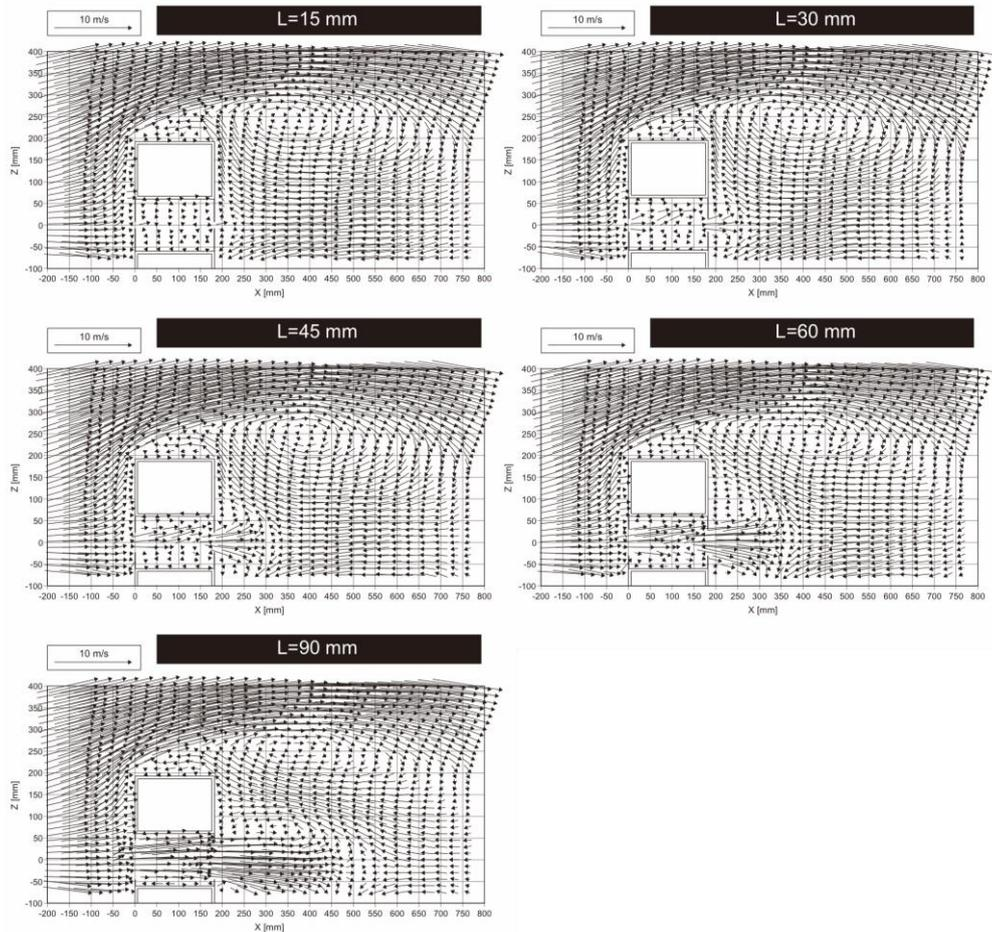
**Fig.7.** Velocity Vector Plots obtained from PIV
