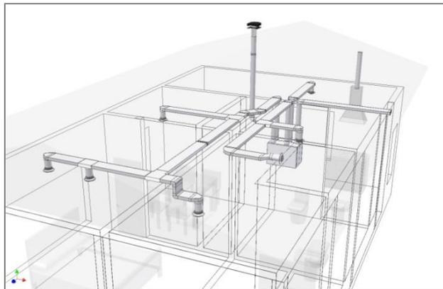
Figure 4: Rectangular thermoplastic ductwork application
