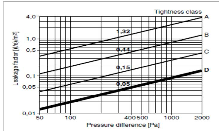
Figure 6: Tightness class according to EN 12237
