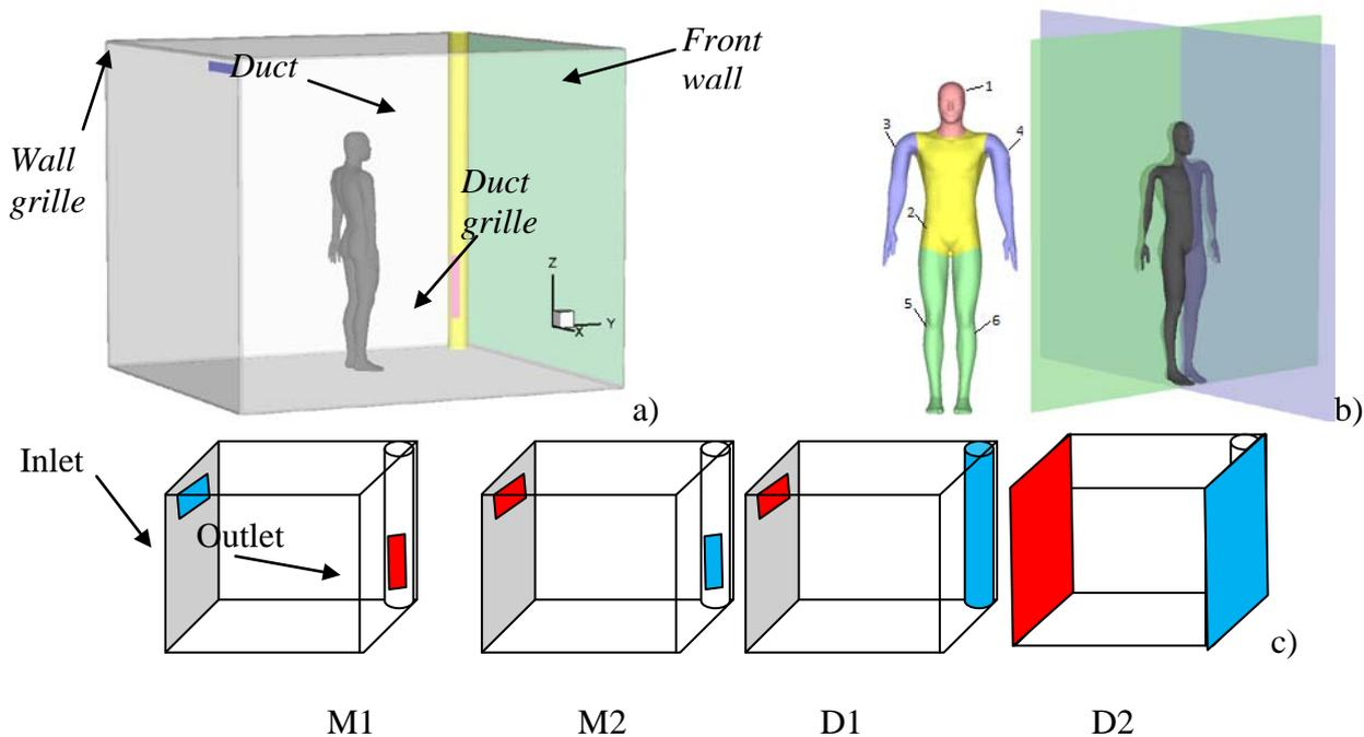
Fig.1: a) Possible inlets in the test cell, b) Human body parts: 1- Head, 2- Torso, 3-Right arm, 4-Left arm, 5-Left Leg, 6- Right Leg, sagittal plan (purple) and coronal (green)c) Inlet and Outlet definition for the four studied cases
