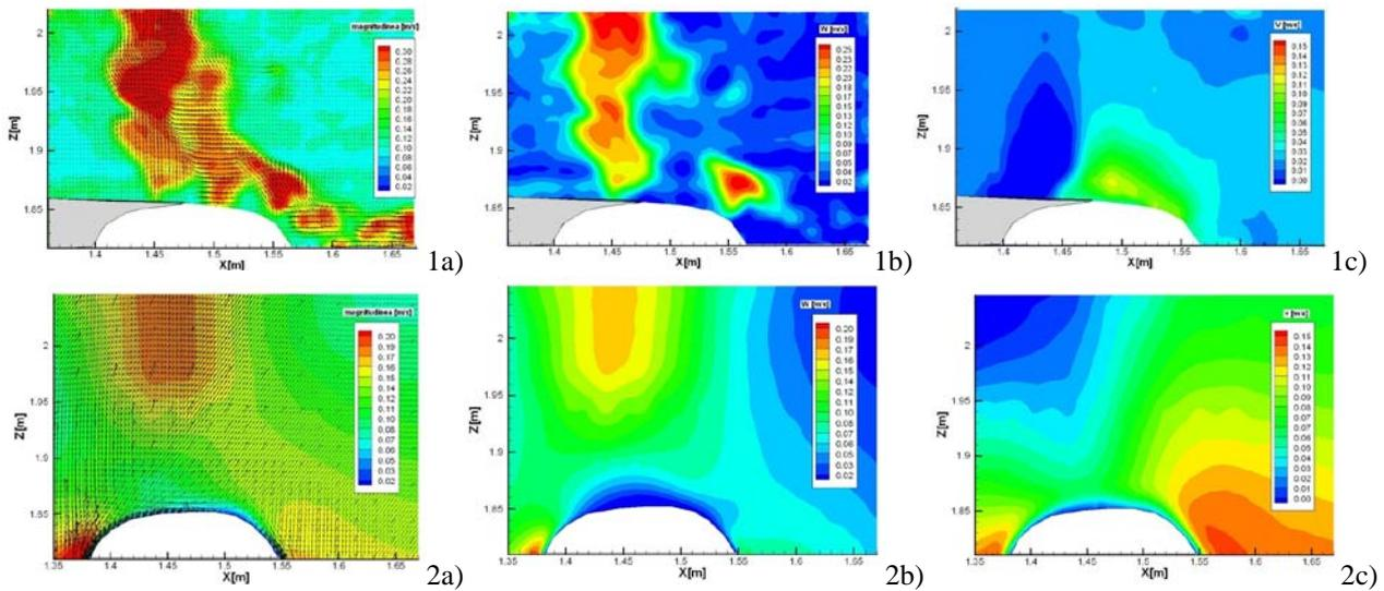
Fig 3. Velocity field comparison –sagittal plan- with jet ( $Tu=10\%$ ): 1 – experimental, 2 –numeric
