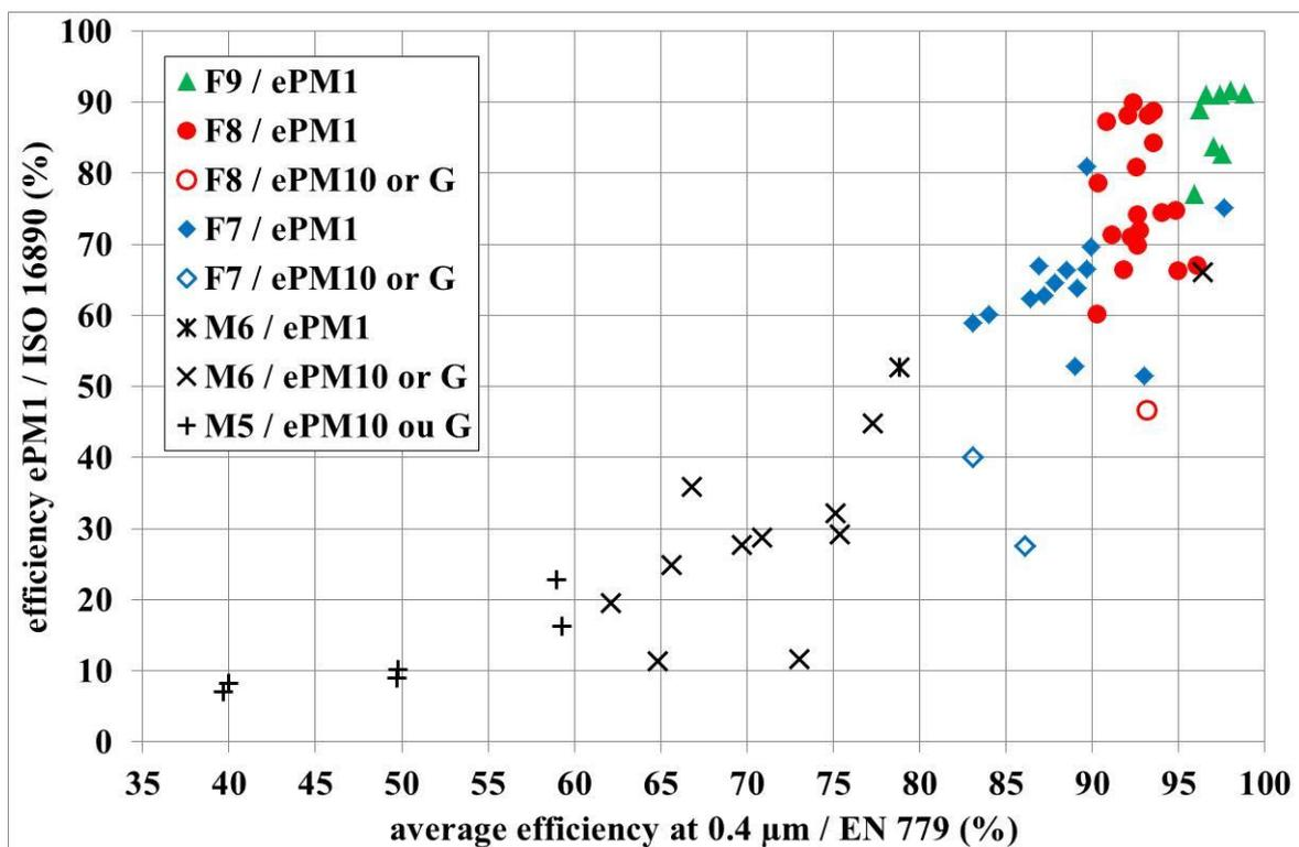
Figure 3: ePM<sub>1</sub> efficiency vs. average efficiency at 0.4  $\mu\text{m}$
