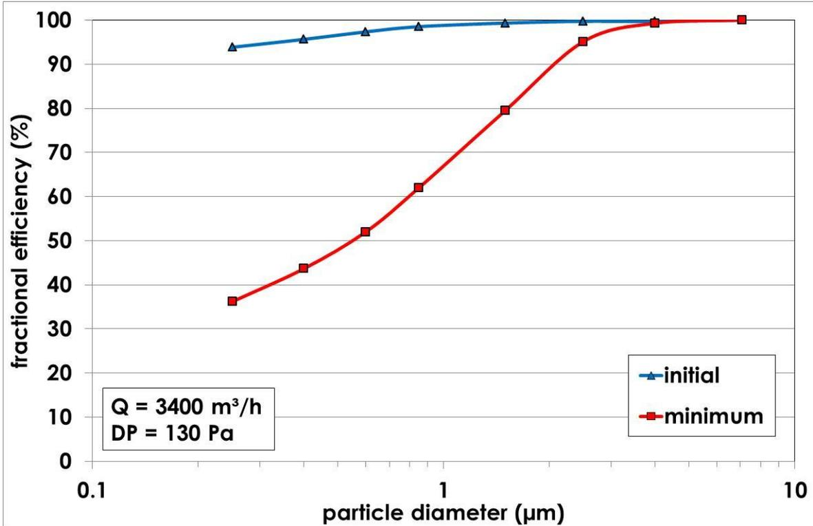
Figure 2: ISO 16890 fractional efficiency test results
