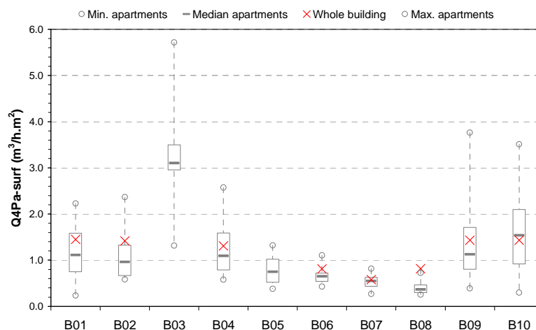
Figure 1: Box plot of the measured air permeability values in each building: the box lines indicate the statistic results of individual measurements and the red marks indicate the measurement of the whole building in each case. The whole measurements of B03* and B05* have been excluded.
