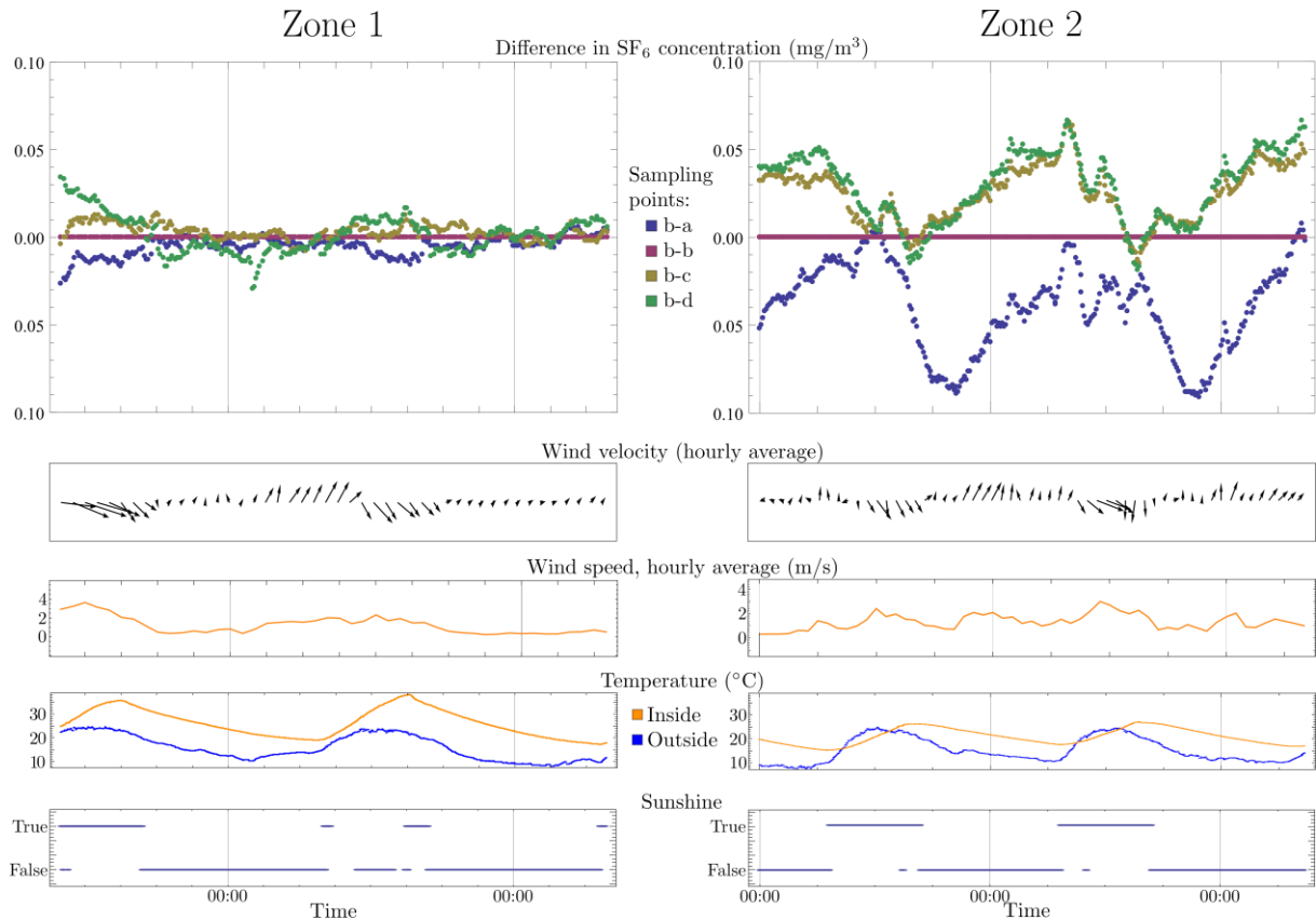
Figure 3: Results of horizontal mixing experiment for Zones 1 and 2. Four sampling points were used in each zone as illustrated in Figure 1(b). A consistent SF 6 concentration across all sampling points in Zone 1 indicates good mixing in the horizontal plane within that zone. Variation in tracer gas concentration at different sampling points in Zone 2 suggests incomplete mixing within that zone.
