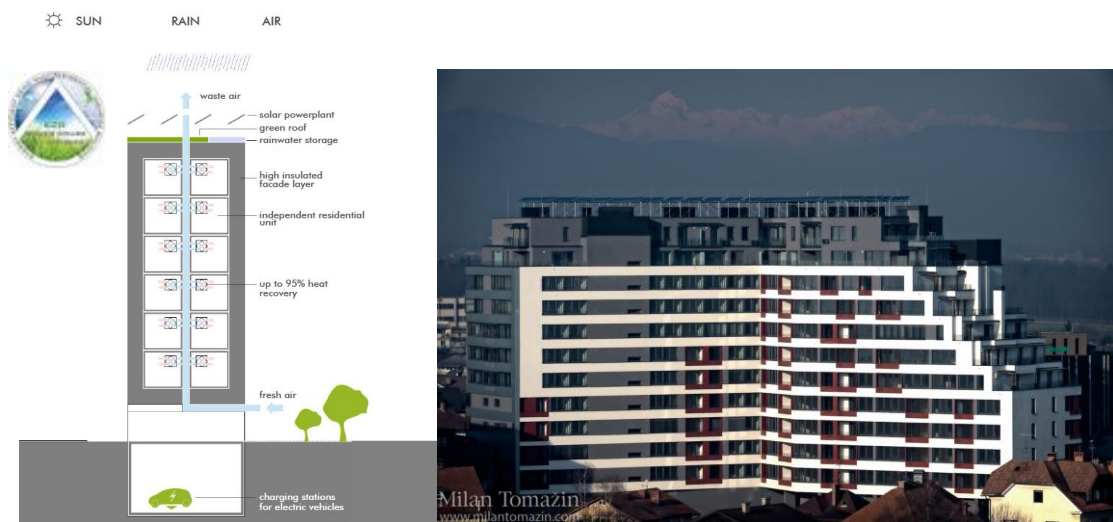
Figure 1: Eco-Silver House – the design concept and the completed building (Design: Akropola; Photo: Milan Tomazin).
