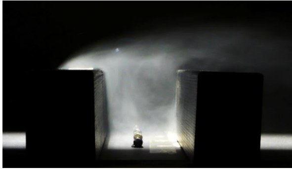
Fig. 8 Line source of emission in the street canyon when F_C=1.0
