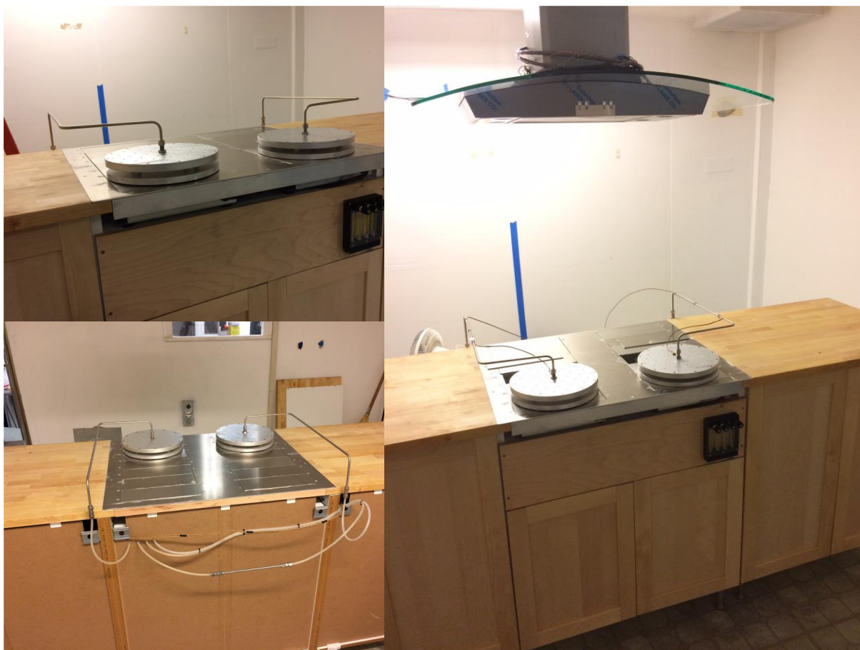
Figure 1b: Island in test chamber showing cabinets, cooktops and overhead range hood
