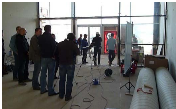
Figure 9: During the BlowerDoor test in the building “Public”
