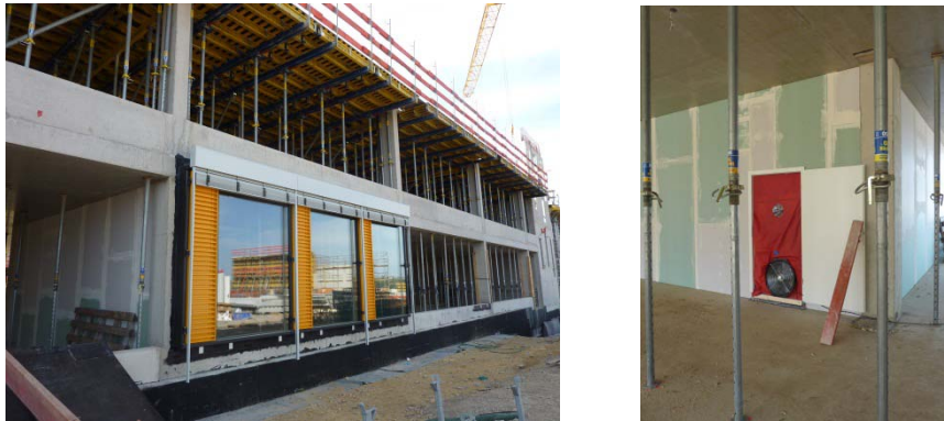
Figure 5: A sample façade with connected casing allowed the airtightness of the façade component and the connecting joint to be tested before construction. In this case, improvements and a second airtightness test were necessary.
