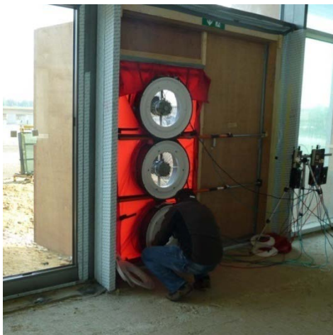
Figure 9: During the BlowerDoor test in the building “Public”
