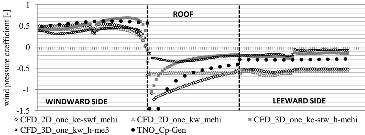
Fig. 3. Comparison of  $C_p$ -values: one opening (CFD), closed building (TNO)
