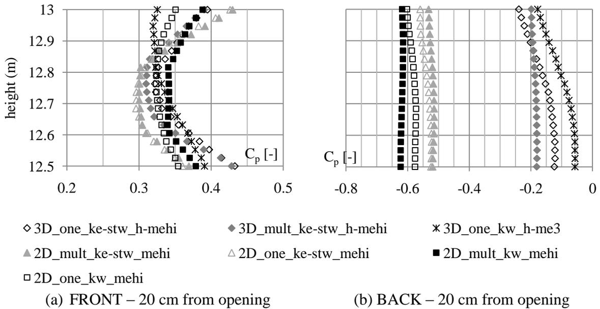
Fig. 6: Comparison of  $C_p$ -profile at opening
