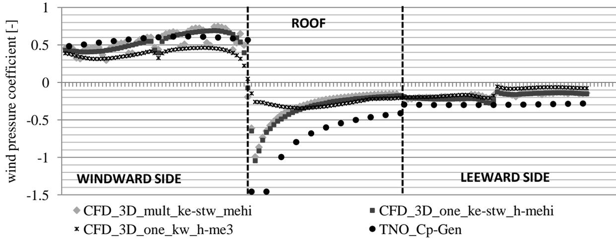
Fig. 5. Comparison of  $C_p$ -values: closed versus one or multiple openings (CFD\_3D) and closed building (TNO)
