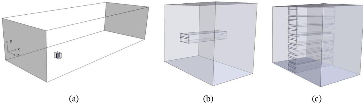
Fig. 1. Overview of (a) building in flow domain and 3D model of the building with (b) one and (c) multiple openings
