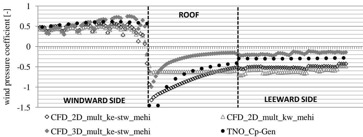
Fig. 4. Comparison of  $C_p$ -values: multiple openings (CFD), closed building (TNO)
