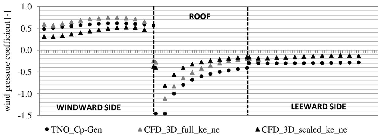
Fig. 2. Comparison of  $C_p$ -values between full scale and scaled model of closed building: verification with TNO  $C_p$ -Generator
