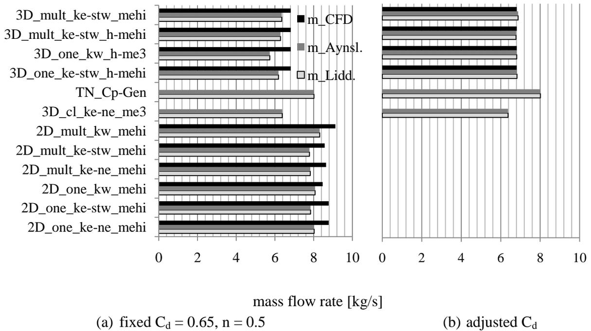
Fig. 8: Comparison of resulting mass flow rates – according to CFD or to approximation formulas
