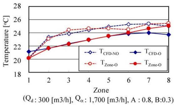
**Figure 10** Comparison between temperature of zonal model results and that of CFD results on each zone ( $Q_\alpha=1700$ ,  $Q_d=300$ ,  $A=0.8$ ,  $B=0.3$ )
