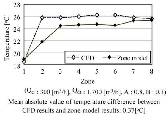
**Figure 11** Comparison between return air temperature of zonal model results and that of CFD results
