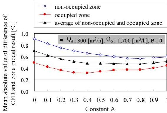
**Figure 8** Mean absolute value of temperature differences  $\Delta T_{(1700, 300, A, 0)}$  between CFD results and zonal model results for all zones when constant A is changed from 0 to 1 at 0.1 intervals ( $B=0$ )
