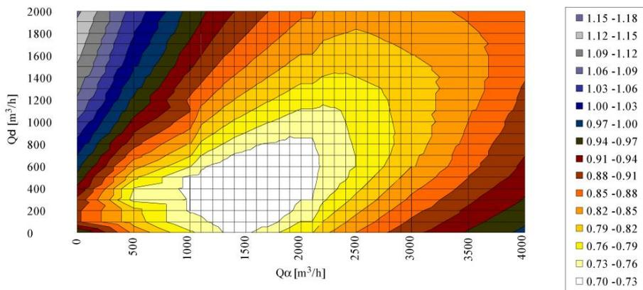
Figure 7 Mean absolute value of temperature differences  $\Delta T(Q_\alpha, Q_d, A, B)$  between CFD results and zonal model results for all zones by combining  $Q_\alpha$  and  $Q_d$  (constant  $A=0, B=0$ )
