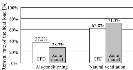
**Figure 12** Comparison between removal rate of heat load by air-conditioning and that by natural ventilation
