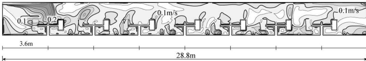
**Figure 3** Distributions of velocity at A-A' Section [m/s]
