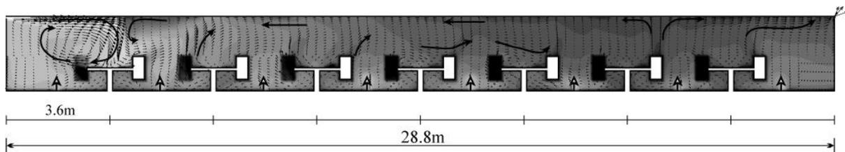
**Figure 4** Distributions of velocity vector and temperature at A-A' Section
