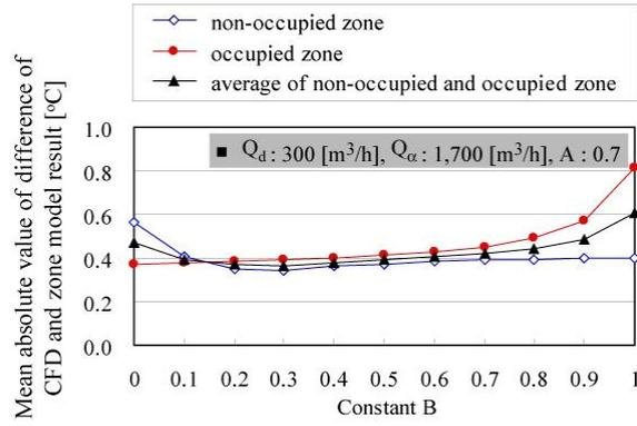
**Figure 9** Mean absolute value of temperature differences  $\Delta T_{(1700, 300, 0.8, B)}$  between CFD results and zonal model results for all zones when constant B is changed from 0 to 1 at 0.1 intervals
