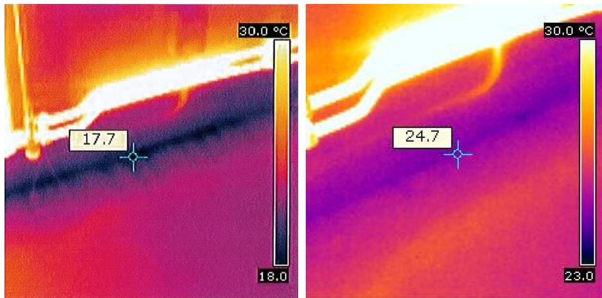
Figure 4: Thermograms showing air leakages in an apartment on the 2<sup>nd</sup> floor along the floor to wall connection before (left) and after (right) the retrofitting. The air leakage is less after the retrofitting (Svensson, 2010, 2011).
