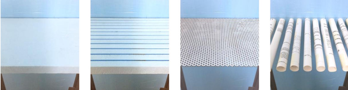
Figure 3: Testes types of obstacles: solid panel, slotted panel, perforated plate, tubes (from left to right)
