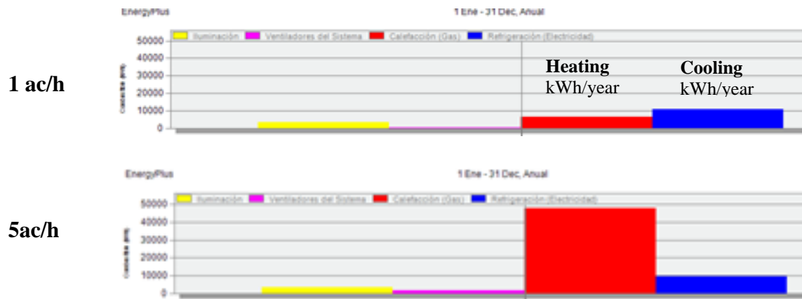
Figure 10: Energy consumption (kWh/year) simulated for one year in Madrid with 1 and 5 air changes per hour . (Red colour: energy for heating; Blue colour: energy for cooling)
