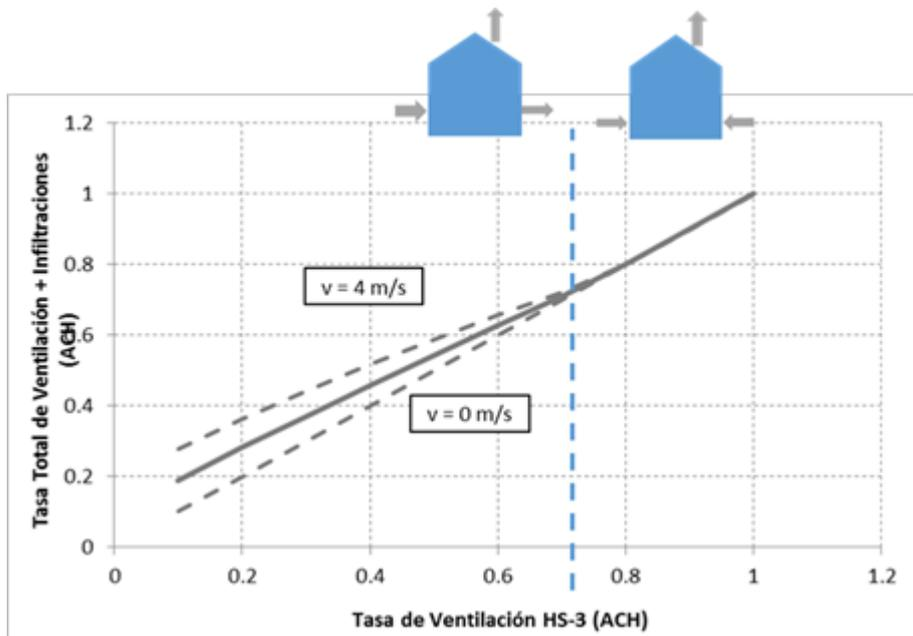
Figure 4: Relation between ventilation + infiltration rate and ventilation rate
