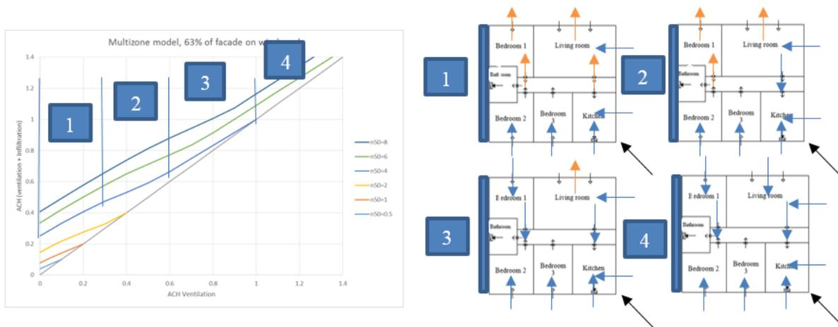
Figure 11: Variation of air flow direction in each facade with  $ACH_{vent}$  for  $n50$  equal to 4
