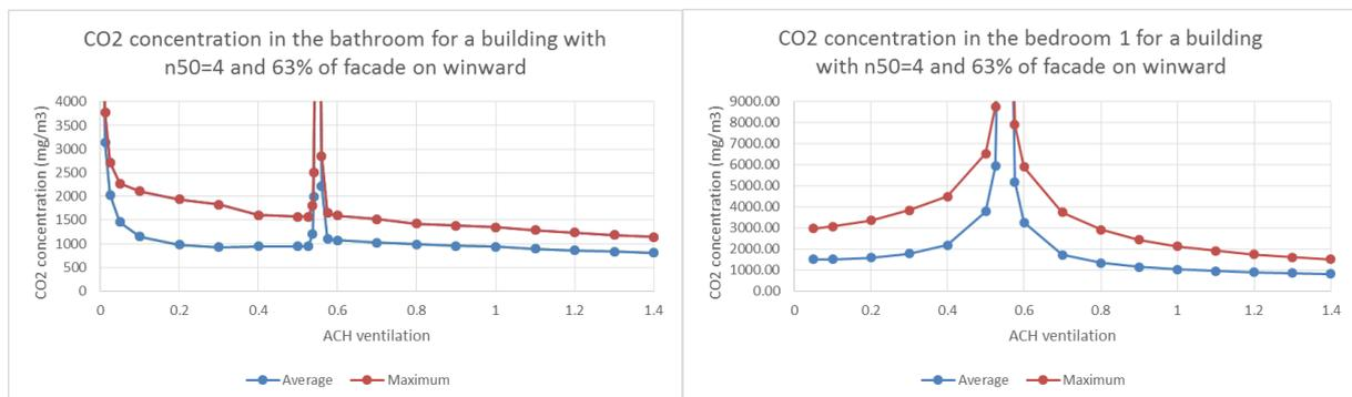
Figure 15: Average (blue) and maximum (red) CO<sub>2</sub> concentration in the bathroom (left) and bedroom1 (right) for a building with n<sub>50</sub>=4 and 63% of façade on windward
