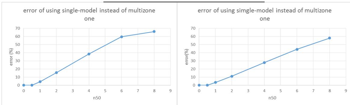
Figure 13: Evolution of maximum error made using a single model instead of a multizone one for 37% (left) and 63% (right) of façade on windward
