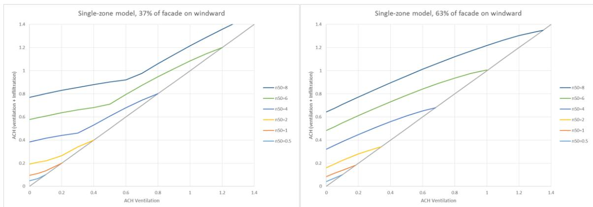
Figure 8: Variation of  $ACH_{vent+inf}$  with  $ACH_{vent}$  and airtightness using the single-zone model with 37% of façade on windward (left) and 63% of façade on windward (right)
