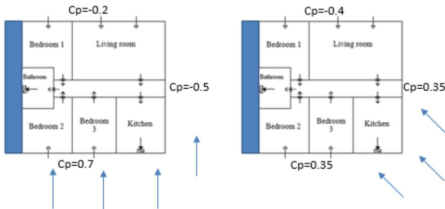
Figure 7: Building with 37% of facade on windward (left) and 63% on windward (right)
