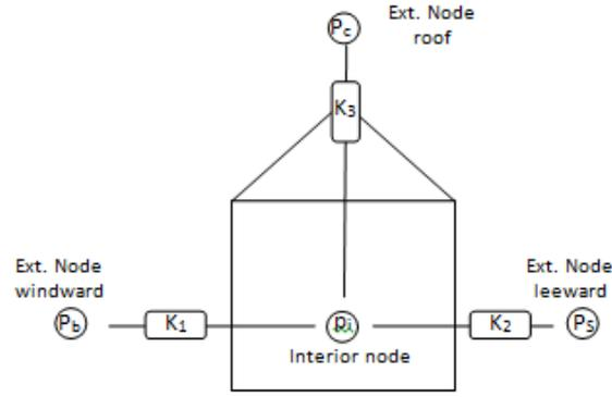
Figure 1: Network nodes in single-zone model
