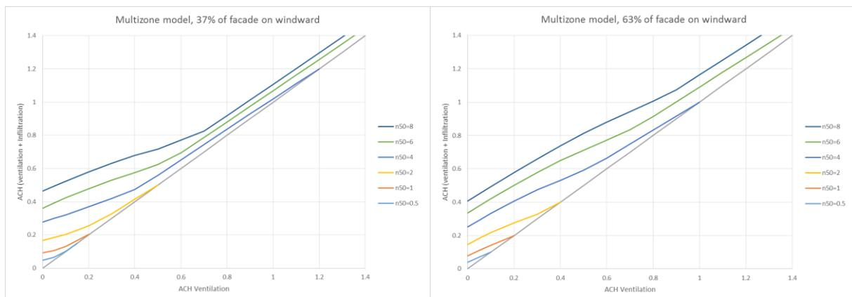
Figure 10: Variation of  $ACH_{vent+inf}$  with  $ACH_{vent}$  and airtightness using the multizone model with 37% of façade on windward (left) and 63% of façade on windward (right)
