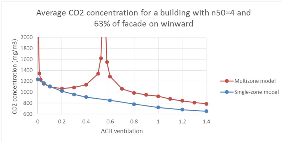
Figure 14: Average CO<sub>2</sub> concentration for a building with n<sub>50</sub>=4 and 63% of facade on windward
