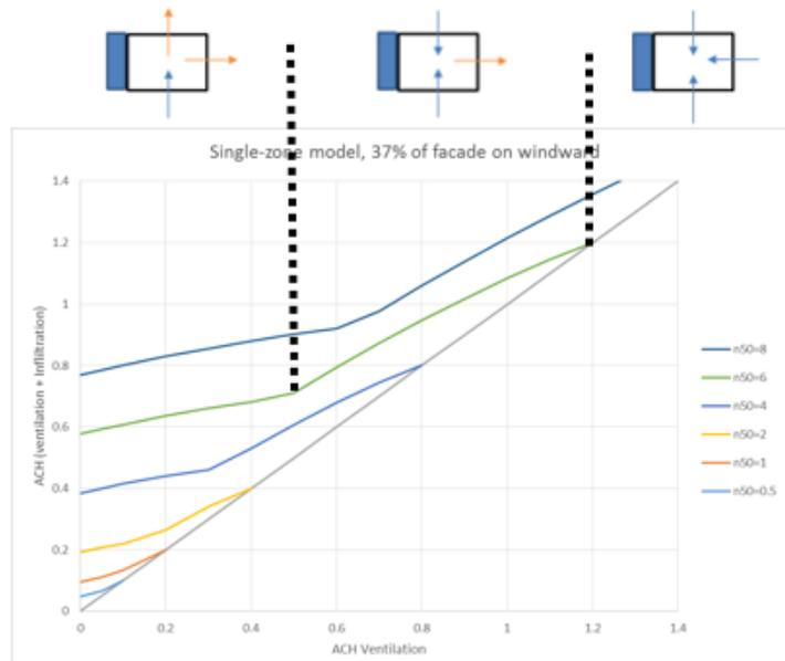
Figure 9: Variation of air flow direction in each facade with  $ACH_{vent}$  for n50 equal to 6
