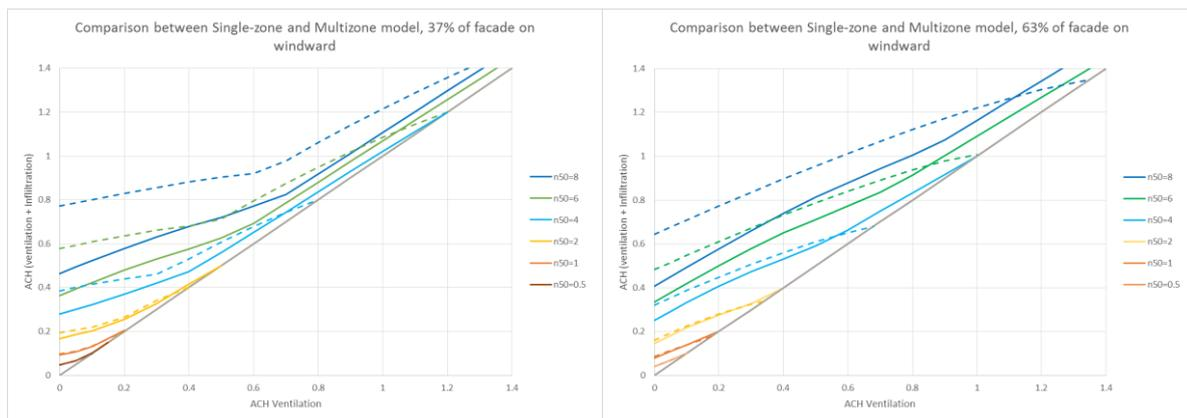
Figure 12: Comparison between single and multizone model for 37% of facade on windward (left) and 63% of facade on windward (right)
