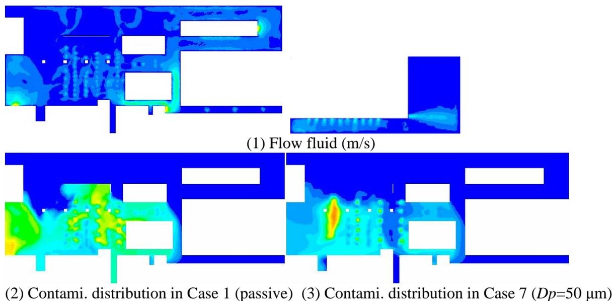
Figure 2 Results of flow fluid and contaminant distribution in hospital ( $y=1.6$  m,  $t=2$  hours)
