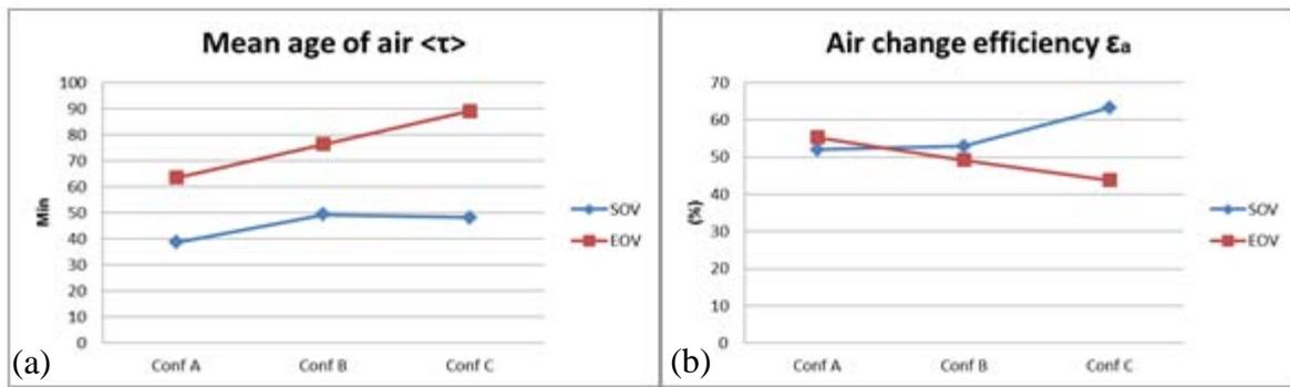
Figure 4-(a) Mean age of air and (b) air change efficiency of the three configurations
