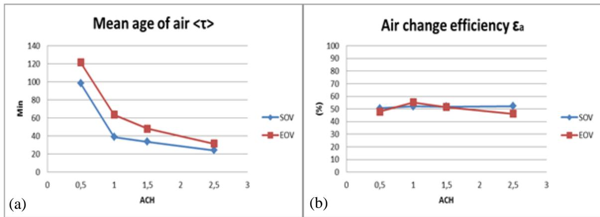
Figure 3-(a) Mean age of air and (b) air change efficiency of configuration A as a function of air change rate
