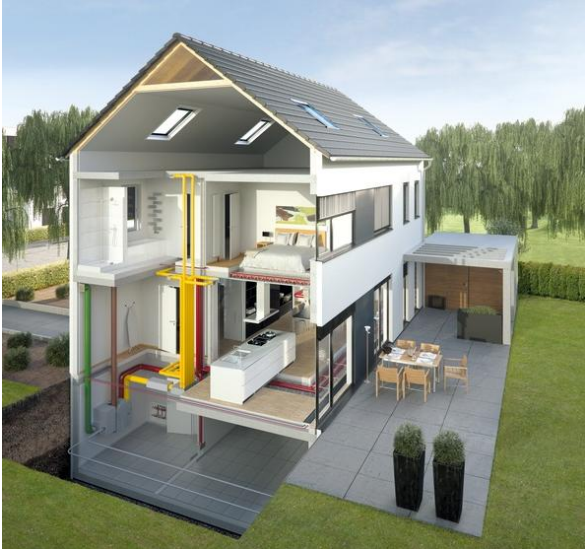
Figure 1: Representation of the ventilation system. Green: outdoor air; Red: supply air; Yellow: extract air; Brown: exhaust air; Grey: the ground collector with glycol-water mixture.
