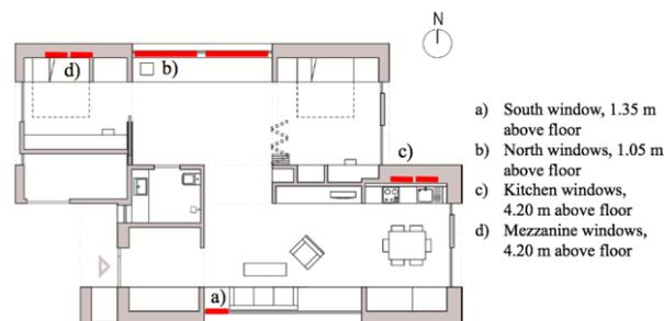
Figure 1. Position of automatically controlled windows in Living Lab (Blandkjenn 2017)
