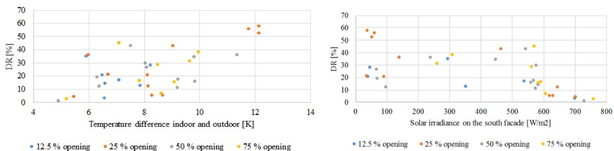
Figure 4 (left) Draught rates as a function of temperature difference, (right) Draught rates as a function of solar irradiance, for different window opening sizes measured in point D (Blandkjenn 2017)
