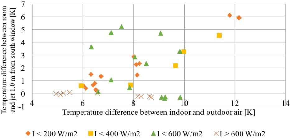
Figure 3. Temperature difference between air in the room and air in the jet 1 m from window, for different levels of solar irradiance.(Blandkjenn 2017)
