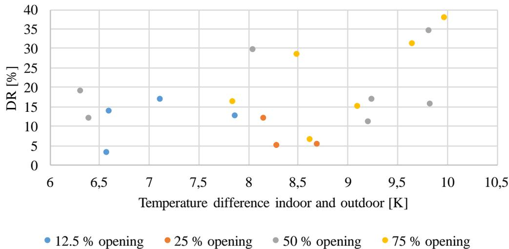
Figure 5. Measurements with  $\Delta T < 10$  K,  $v < 2$  m/s and  $I > 70$  W/m<sup>2</sup> (Blandkjenn 2017)
