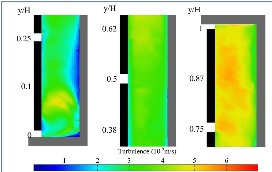
Figure 6: From left to right: turbulence in a middle plane of measurement at three different cavity heights.
