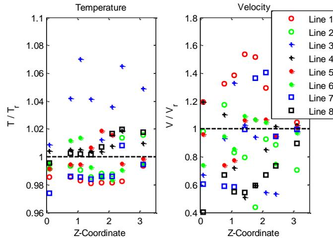
Fig. 3: Ratio of temperatures, one with considering the radiative heat transfer ( $T_r$ ) and one without ( $T$ ) [left]; and ratio of velocities with ( $V_r$ ) and without ( $V$ ) considering the radiative heat transfer [right]
