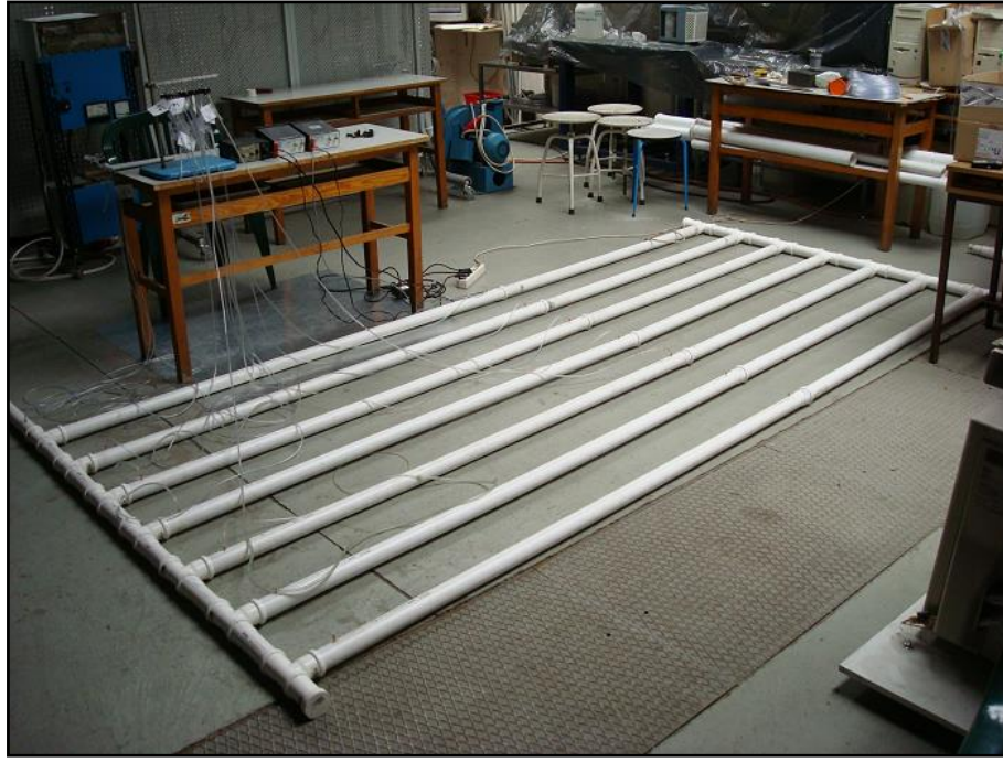
Figure 3: View of the experimental set-up: Z-type, 7 pipes 90° EAHE model in a scale 1:4
