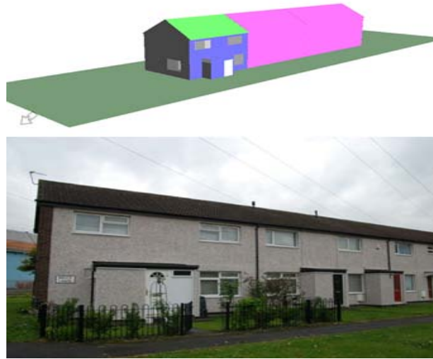
Figure 5. Case study of the end-terraced house in Leeds and the model built in IES VE.
